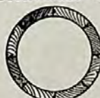
* CROSS SECTION OF HOLLOW SPAR *
